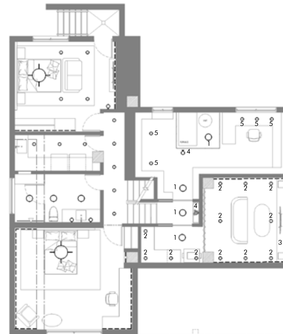
Reflected Ceiling Plan
