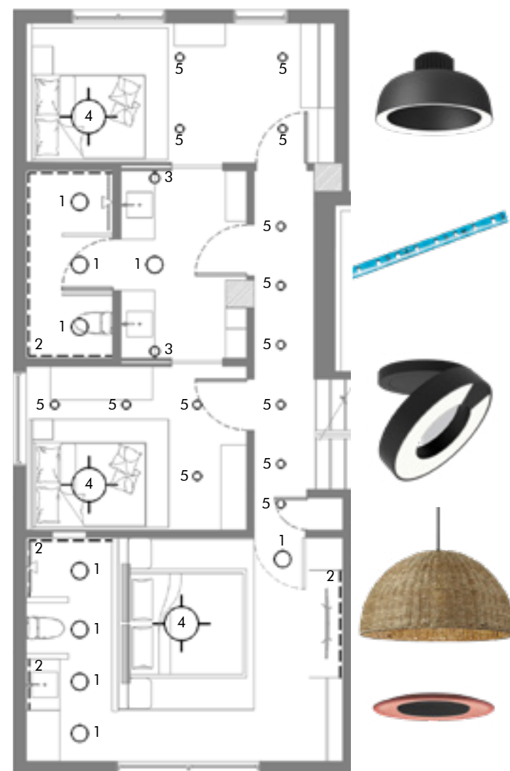
Reflected Ceiling Plan
